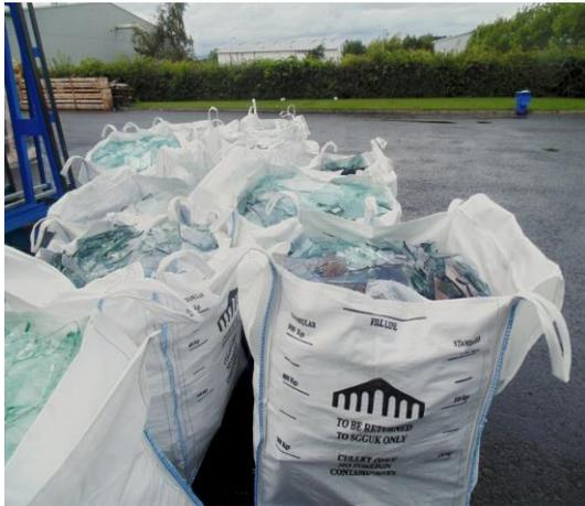
The scheme from Saint-Gobain Glass UK, enables the utilisation of over 30% recycled material in the manufacture of float glass. The scheme enables waste to be diverted away from the landfill and leads to fewer lorries on the road, whilst using less energy as well as fewer raw material in the manufacturing process. This all helps towards producing less of the greenhouse gas CO<sup>2</sup>.
