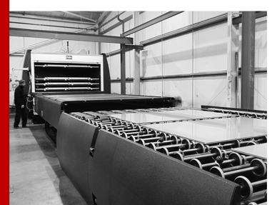
Our structural glass is toughened in accordance with BS EN 12600 with options including clear or tinted with the option of acid etching.
